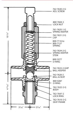
**APPLICATION:** Recommended for overpressure protection where buildup and blowdown must be held to a minimum. Designed to meet all protection requirements for gathering lines, transmission systems, meter runs, gas manifolds, separators and refinery service.
