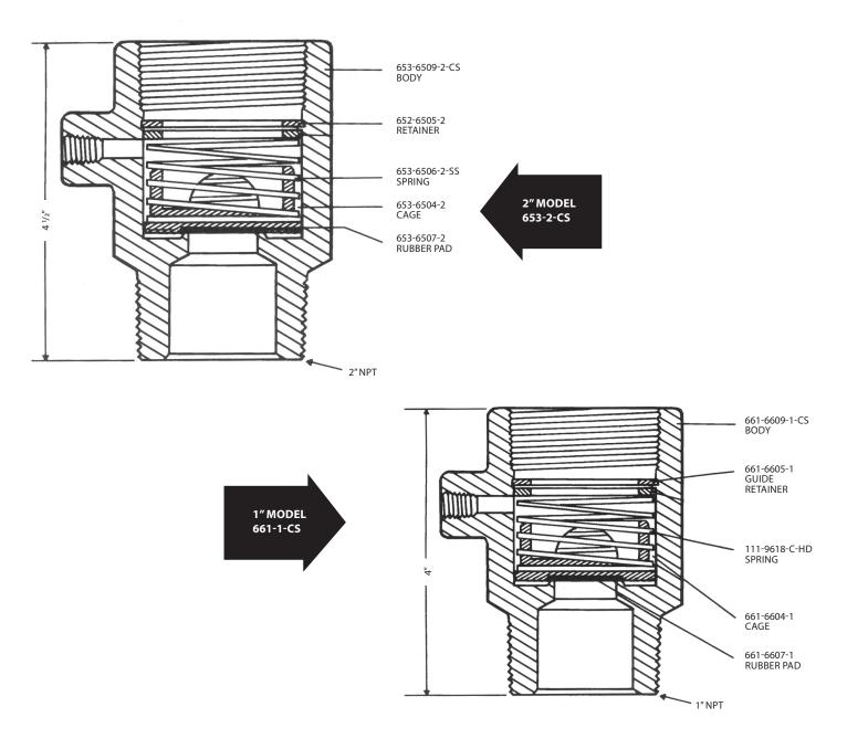
Baird VALVE CHECKER: Installed in front of the safety valve inlet, permits the operator to monitor valves with periodic pressure checks. This gives assurance that the valve is relieving properly at the set pressure, and reclosing as it should.
