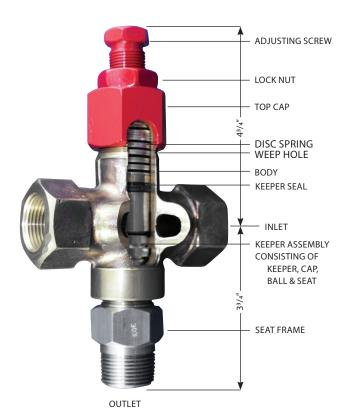
This valve was designed for pumping through one side and out the other with a built-in relief. By tying the ball to the keeper, the over-pressure simply lifts the whole spring assembly with a diaphragm action allowing relief out the bottom.
