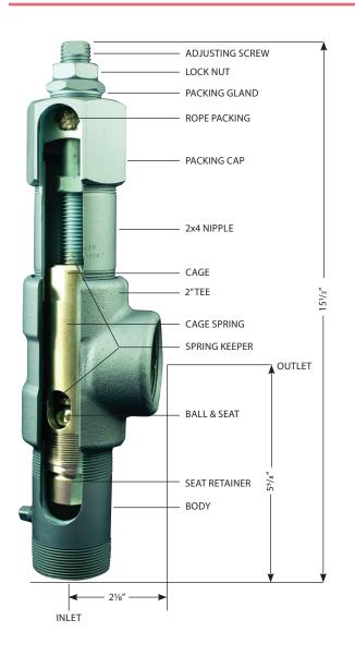
The Baird "Old Style" BPR<sup>®</sup> was made in 1950. Ever since that time, the Baird Back Pressure Regulator has been universally accepted by the oil and gas industry as a sure solution to a variety of production problems. As a result, it is widely stocked in oil field supply stores.
