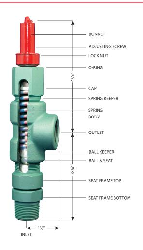
Designed as an inexpensive 1" steel pressure control valve. **May** be used as a relief or back pressure valve. This valve was patterned from our 7100 1" gas valve, but the ball and seat are more durable for more severe liquid service. May also be used for gas.
