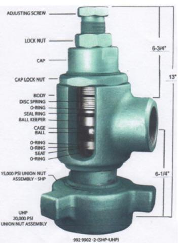
Designed for protection against over-pressure for pumps. It is a rugged and versatile valve capable of handling a wide range of pressures.
