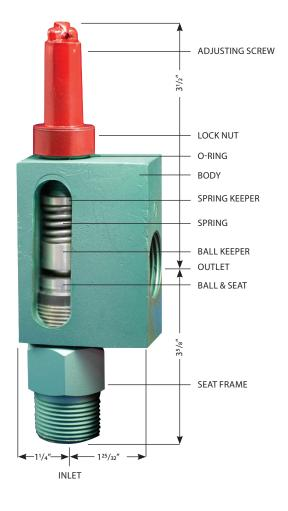
A rugged, economical valve for low pressure, low volume applications. It is adjustable and repairable in the field or in the line.
