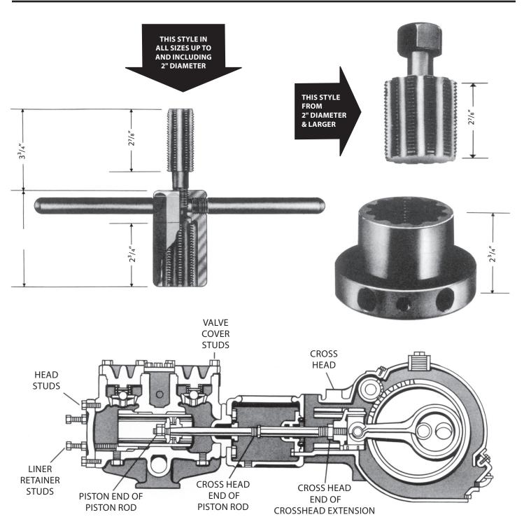
API Taper Number for Piston End of Piston Rod on Slush Pumps (See price list on page 27).
