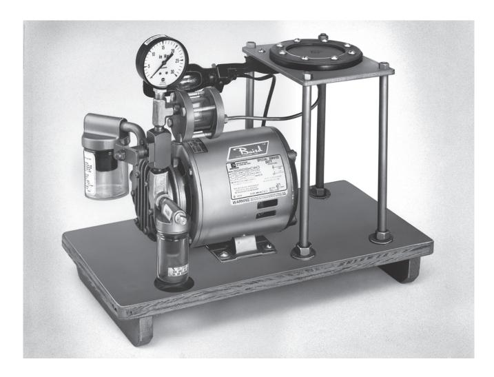
A conventional ball and seat is one of the least expensive parts in the repair of a pump, yet one of the most important. Many times a visual inspection can find nothing wrong with the ball and seat, but a test will prove the assembly to be defective beyond a doubt. Because the efficiency of the pump is completely dependent upon the effective seal in the ball and seat, always insist that your assemblies be tested with the Baird bubble type tester.
